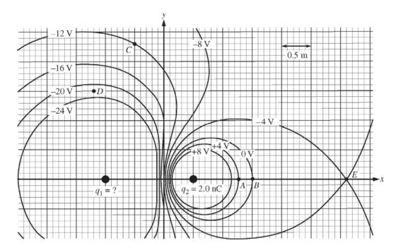
Two point charges,  $q_1$  and  $q_2$ , are fixed in place on the x-axis at positions  $x_1 = -1.00$  m and  $x_2 = +0.50$  m, respectively. Charge  $q_2$  has a value of +2.0 nC. Values of electric potential are illustrated by the given equipotentials in the diagram shown above, which is drawn to scale.
